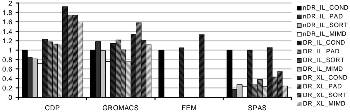
**Figure 7: Computation cycle simulation results for all mapping variants across the four applications. Execution cycles measured with perfect off-chip memory and normalized to the nDR\_IL\_COND variant of each application.**
