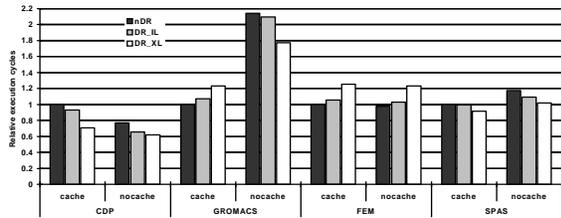
**Figure 8: Performance results for the best performing parallelization variant of each application with a realistic memory system. The *cache* configuration employs a stream cache, while *nocache* dedicates more on-chip memory to the SRF.**
