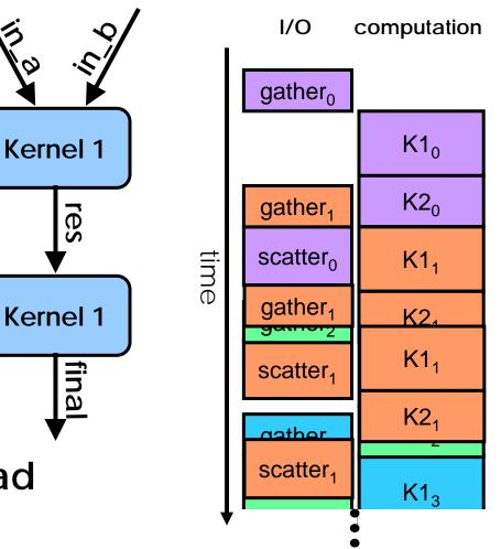
Hardware designed for throughput and not latency (memory BW, FLOPS, bulk exceptions, bulk coherency, ...)
