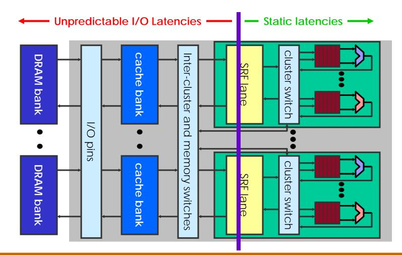
Decoupling enables efficient static architecture Separate address spaces (MEM/SRF/LRF)
