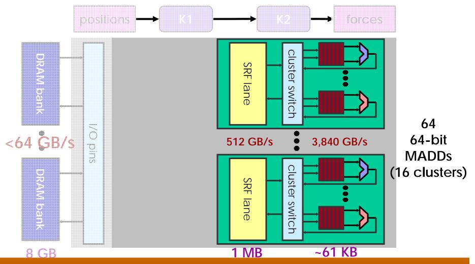
SRF reduces off-chip BW requirements (producerconsumer locality); enables latency-tolerance
