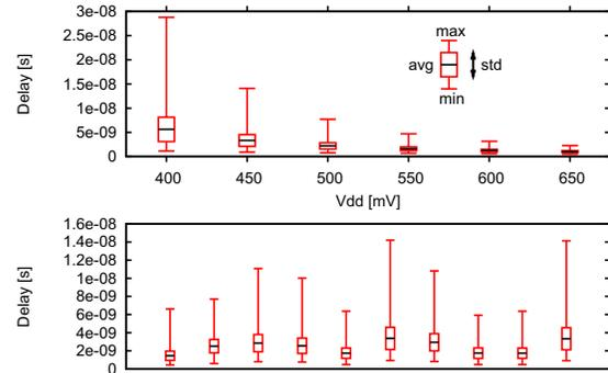
Fig. 2: Results of random-dopant fluctuation Monte Carlo experiments for delay of a 16-bit multiplier ( $90nm$ ,  $V_{th}=0.4V$ ): worst-case delay as function of  $V_{dd}$  (top) and delay of 10 random input vectors at  $V_{dd}=0.45V$  (bottom)
