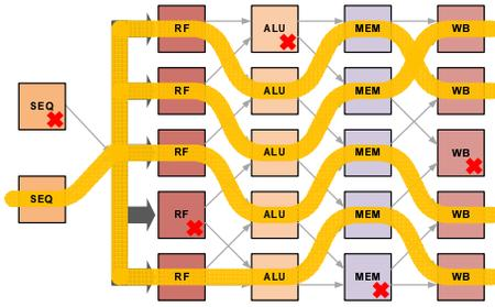
Fig. 5: Weaved-pipeline sparing for DPSP and SIMD PEs. Shared pipeline components are replicated once and, in this example, a sparing of  $\frac{1}{4}$  is added to the parallel SIMD path. Components that failed testing are marked with an X and are disabled along with their wires.
