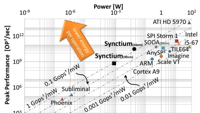
Fig. 1: Power and performance ( $\dagger$  normalized to 16-bit operations) of a range of processors showing the need for a relatively high-performance  $\sim 1mW$  processor.  $\ddagger$  AnySP numbers are from fig. 14 in [19].
